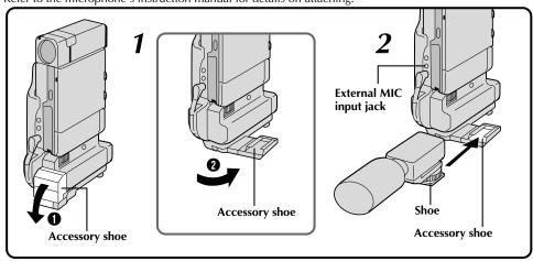
Insert the microphone's shoe into the accessory shoe. Then connect the microphone's ø3.5 mm mini-plug connector to the external MIC input jack on the camcorder.
