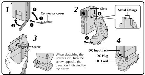
Remove the camcorder's connector cover as indicated by **1**, **2**.
