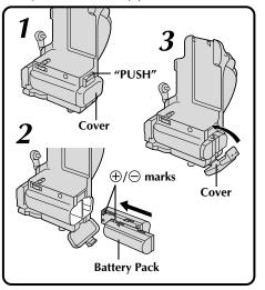
Press down "PUSH" and open the cover in the direction of the arrow.
